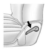
On vehicles with seats that have manual reclining seatbacks, the lever used to operate them is located on the outboard side of the seat.
